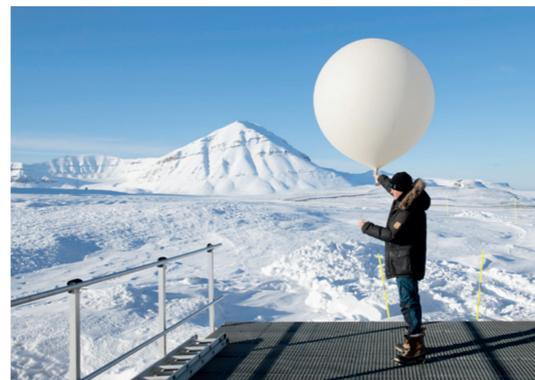
Launch of a radiosonde for atmospheric measurements. (Photo: AWIPEV / E. Horvath)
