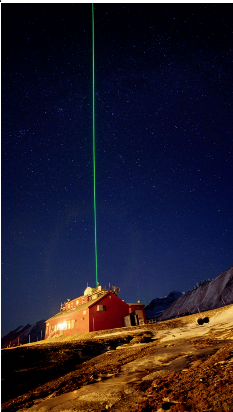
The atmospheric observatory with the green laser beam of the lidar system, which measures the aerosol distribution in the atmosphere. (Photo: AWIPEV / R. Bürgi)
